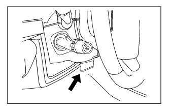
To tilt and telescope the steering wheel, pull down the lever. Then move the steering wheel up or down or backward or forward into a comfortable position. Pull the lever up to lock the steering wheel in place.
